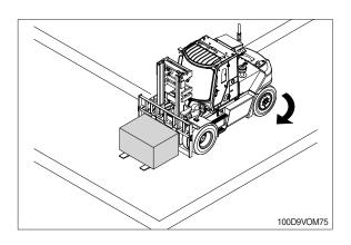
▲ Turn too sharp with a raised load and your truck can tip even at slow speeds. Travel with a load raised only when removing or depositing a load.
